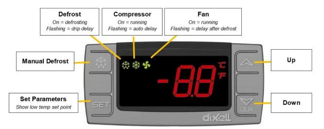
To see your set temperature, press and release "**SET**". To change it, hold "**SET**" until **F** is flashing and use up or down to adjust. This temperature must be within the selected temperature range in the parameters. To check or adjust the parameters, follow the steps below.
