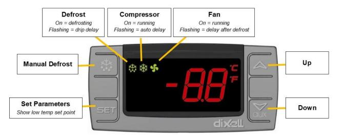
To see your set temperature, press and release "**SET**". To change it, hold "**SET**" until **F** is flashing and use up or down to adjust. This temperature must be within the selected temperature range in the parameters. To check or adjust the parameters, follow the steps below.
