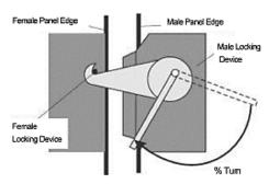
Assemble floor panels first, followed by wall panels. Assemble wall panels starting at circle and continue in the direction of arrows. Add door frame then roof panels. Apply included sealant at all joints.
